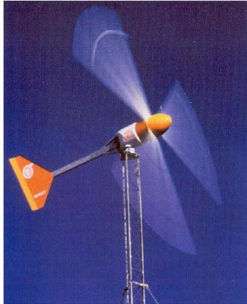
Figura 4.1 – Turbina Bergey Excel 7,5 kW.
