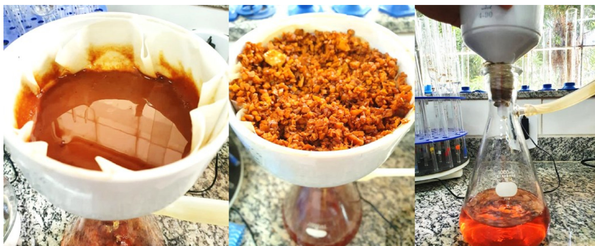
Figure 1. Filtration processing using the vacuum system to separate the extract solid from the extracting solvent after 10 days of maceration
